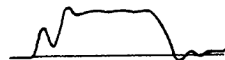
FIG. 3-4.—Delay between the switching waveform and the initiation of r-f oscillations. The buildup of oscillations in a lighthouse tube (2C43) operating with 1000 volts at the plate is shown, indicating a delay of roughly \frac{1}{2} \mu sec. The duration of the current pulse is 1.16 \mu sec.
